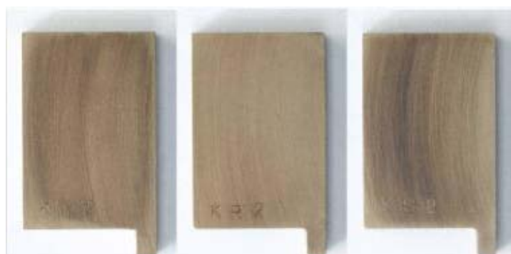
Fig. 1: Example images of coupons made of „compressor steels“ (from left to right: 1.4006, 1.4313, 1.4542) after 600 hours at 170 °C in continuous CO 2 stream at atmospheric pressure.
