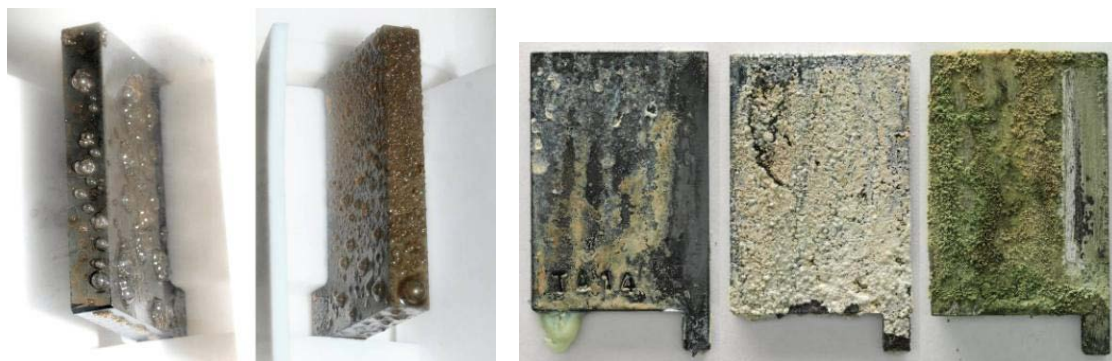
Fig. 4: left: Generation of bubbles on coupon surfaces due to condensation of acids and gas generation at 5 °C and 0.8 % water, 1,8 % oxygen, 760 ppm CO 2 , 1000 ppm SO 2 and 220 ppm SO 2 . right: Corrosion of low alloyed pipeline steels after 120 hours at 5 °C in CO 2 containing 2 % H 2 O, 0.6 % O 2 and 650 ppm SO 2 .
