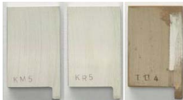
Fig. 3: Example images of coupons (from left to right, 1.4006, 1.4313, 1.1018) after 600 hours at 60 °C in continuous CO 2 stream at atmospheric pressure.
