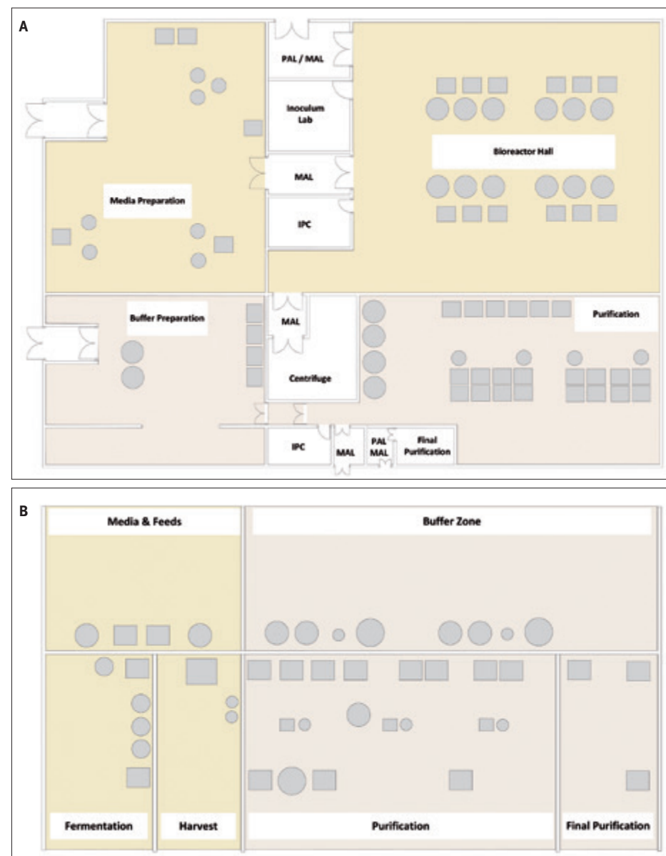
Figure 5: Schematic representation of the “ballroom” concept (A) and the “dance floor” concept (B).
